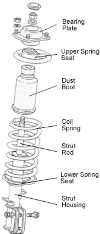
The top of the strut is connected to the vehicle body through the **upper strut mount**, in some cases called **abearing plate**.
