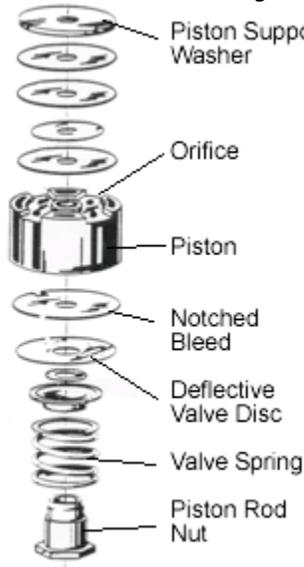
**Bore size** is the diameter of the piston and the inside of the pressure tube. Generally, the larger the unit, the higher the potential control levels because of the larger piston displacement and pressure areas. The larger the piston area, the lower the internal operating pressure and temperatures. This provides higher damping capabilities.
