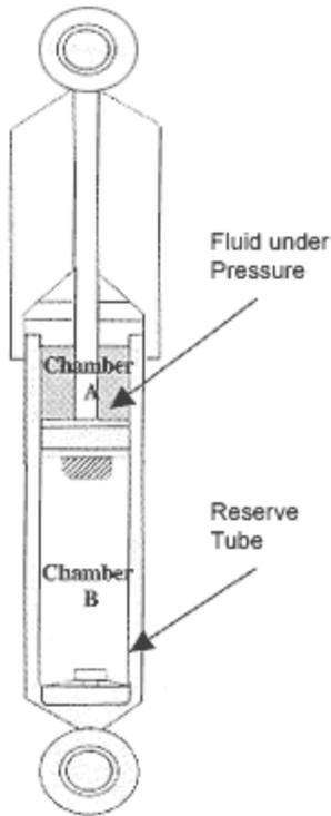
**Extension cycle** As the piston and rod move upward toward the top of the pressure tube, the volume of chamber A is reduced and thus is at a higher pressure than chamber B. Because of this higher pressure, fluid flows down through the piston's 3-stage extension valve into chamber B.
