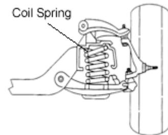
The diameter and length of the wire determine the strength of a spring.
