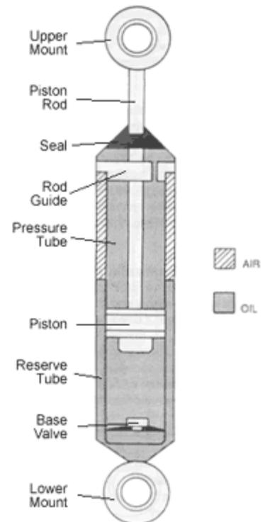
with the pressure tube and allows the piston to move freely inside. The **seal** keeps the hydraulic oil inside and contamination out.
