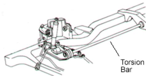
During suspension movement, the torsion bar will twist, providing spring action.
