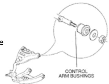
During suspension travel the rubber portion of the bushing must twist to allow control arm movement. Control arm bushings that are in good condition act as a spring; that is, the rubber will spring back to the position from which it started. This twisting action of the rubber will provide resistance to suspension movement.
