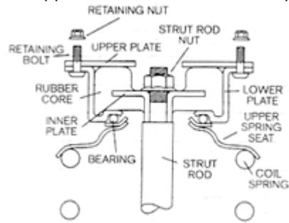
However, these components wear over time and with a thorough inspection a proper recommendation can be made. The bearing is located on the bottom of the strut mount and is not serviceable. Defective bearing will require replacement of the entire strut mount.
