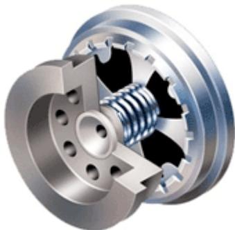
A new twist on the comfort/ control compromise is an innovative technology which provides greater control for handling while improving ride comfort called **Acceleration Sensitive Damping (ASD)**.
