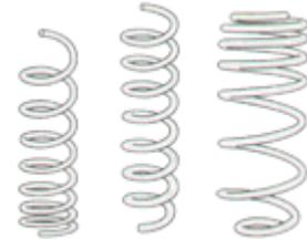
Ride height measurements not within manufacturer's specifications require replacement of springs.
